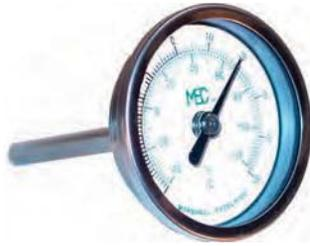
Designed for use in LP-Gas or NH<sub>3</sub> storage tanks, nurse tanks, bobtails and transports. These stainless steel, dust and water proof thermometers feature a 1/2" MNPT connection with a temperature range from -40° to +120° Fahrenheit. Accuracy +/- 1 percent full range.
