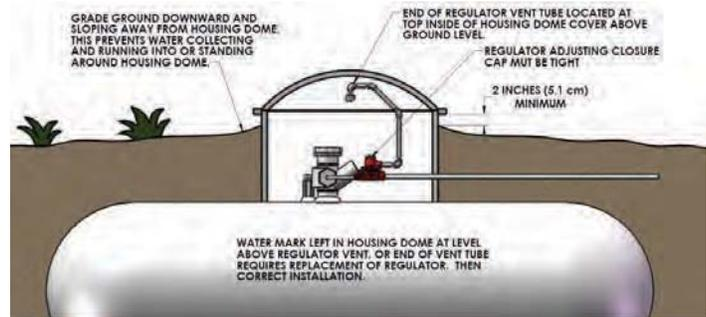
Figure 5: Underground Installation
